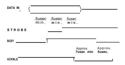
Data must be present a minimum of 0.5 microseconds before and after a minimum 0.5 microsecond STROBE pulse. BUSY goes high before the end of the STROBE signal and remains high until the end of an ACKNLG pulse of minimum 4 microseconds.
